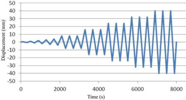
Figure 3 Displacement sequence for the quasi-static cyclic test
