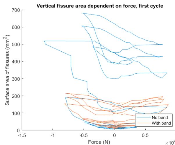
Figure 7 Vertical fissure area in relation to the applied force during the first cycle
