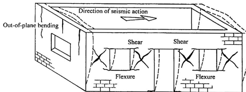
Figure 1 Various failure mode in a masonry structure (Tomažević, 1999)
