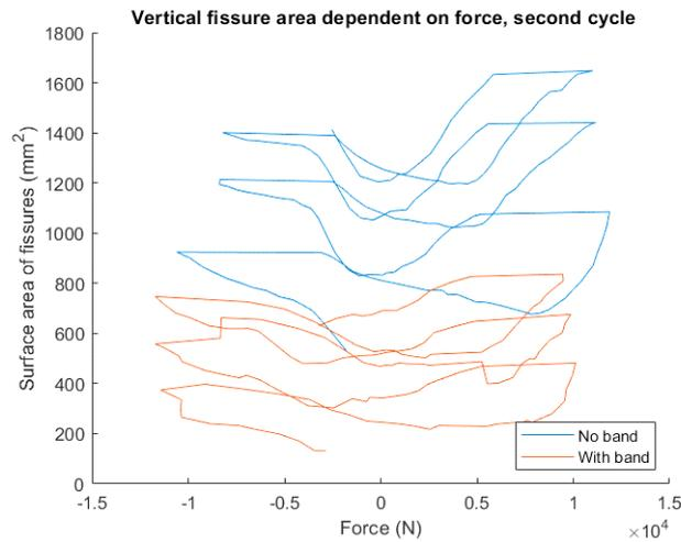
Figure 8 Vertical fissure area in relation to the applied force during the second cycle
