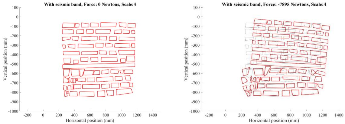
Figure 5 DIC displacement output field for masonry wall with timber band at zero force (left) and 7.89 kN force (right)
