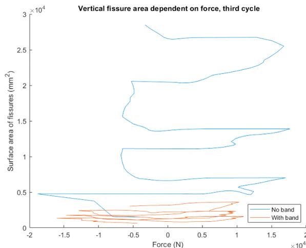
Figure 9 Vertical fissure area in relation to the applied force during the third cycle
