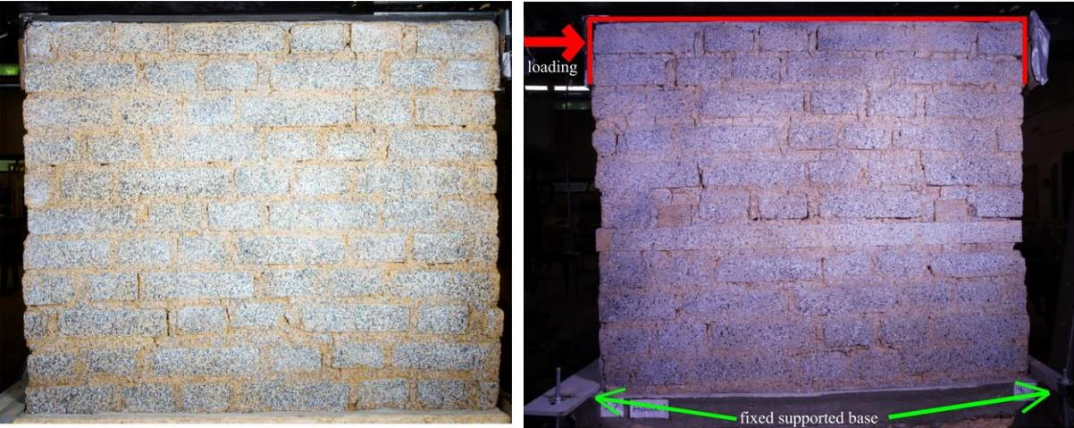
Figure 2 Masonry wall without a band (left) and with timber seismic band (right)
