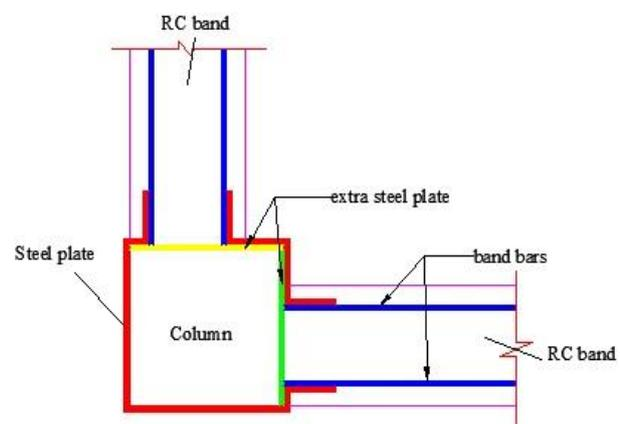
Fig 6. Steel plate as an anchor for RC band
