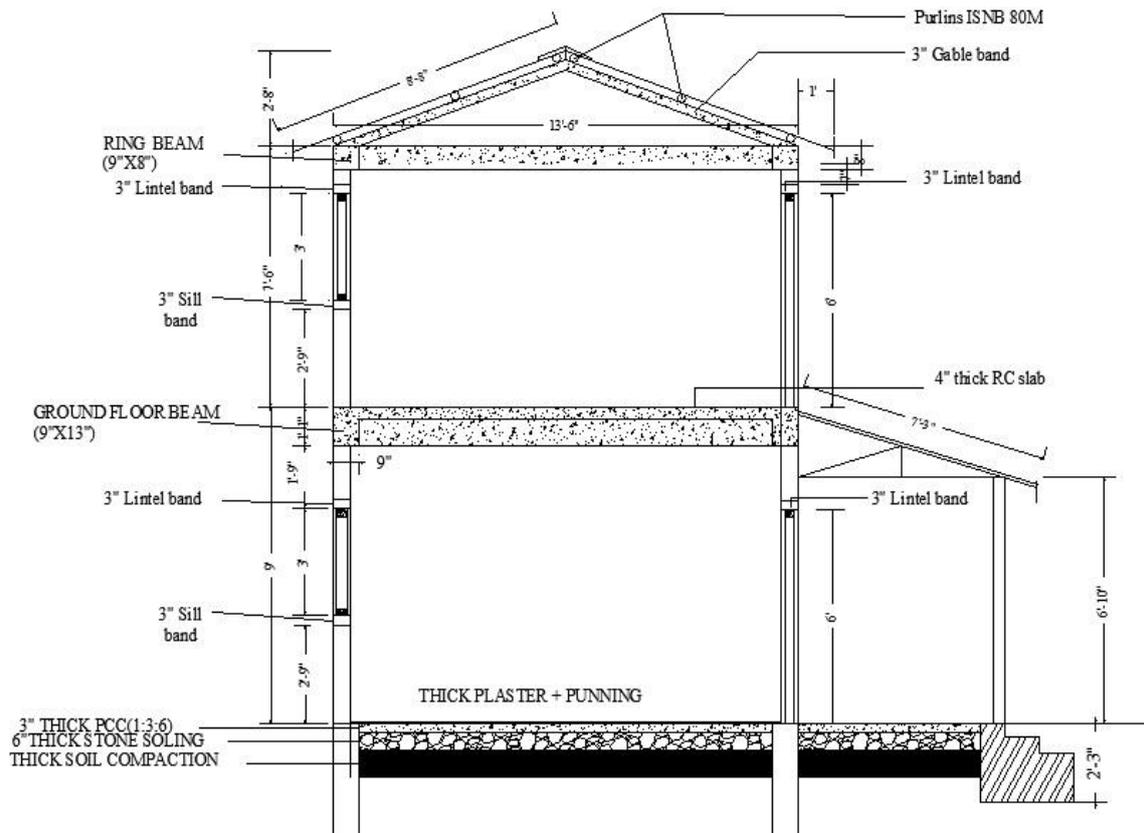
**Fig 3.** Sectional view of the planned building
