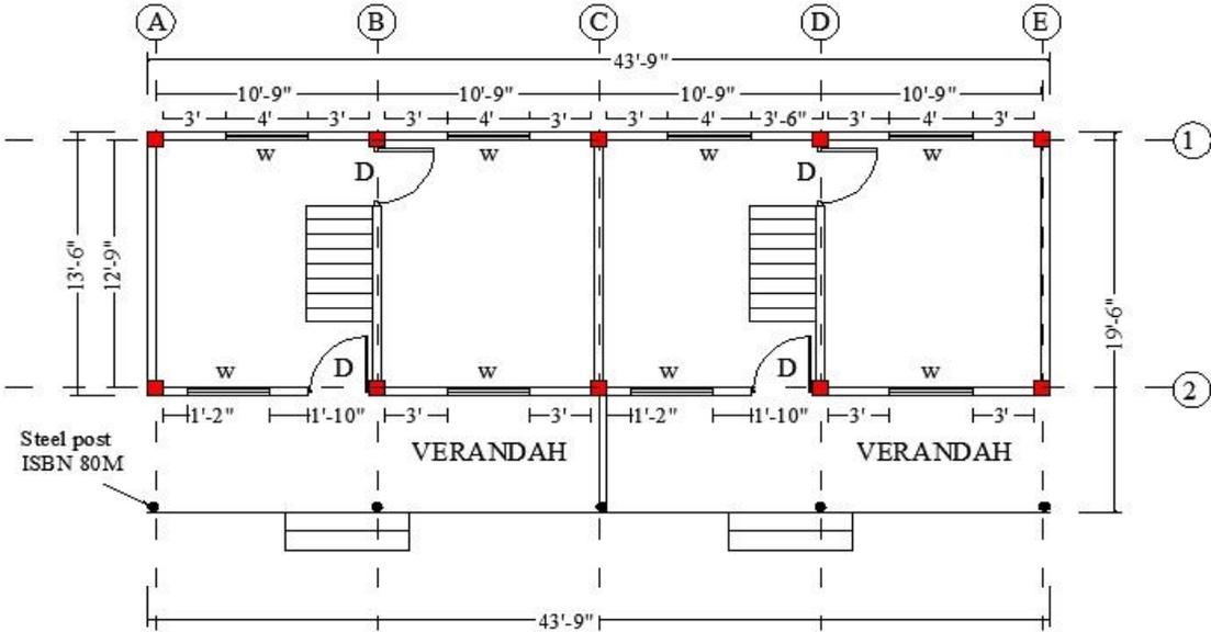
Fig 2. Ground Floor plan for building (dimension in feet-inch)
