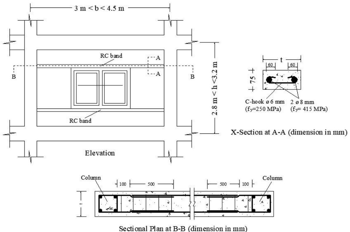
Fig 4. Detail of RC bands at lintel and sill level for infill wall (NBC 201, 1994b)
