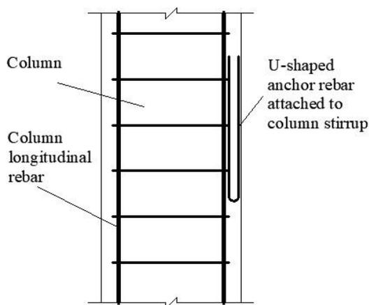
Fig 5. Arrangement of anchor rebar for RC band
